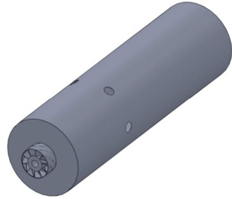
FIGURE 1: The CAD model of combustion chamber
