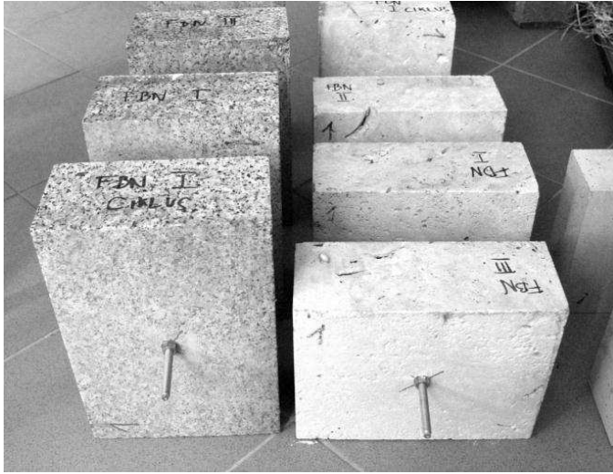
Figure 6. Granite and limestone blocks for pull-out tests
