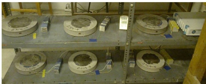
Fig.5. Cement stone ring specimens during the test
