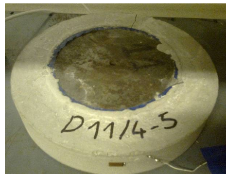
Fig.4. A crack on a ring specimen
